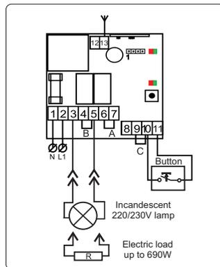
Fig. 3. Scheme that shows how to connect Radio 8113 IP65 to a lighting unit or other electric devices.
