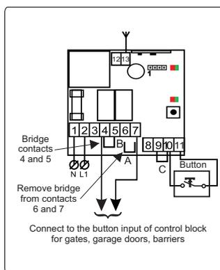
Fig. 2. Scheme that shows how to connect Radio 8113 IP65 to a step-by-step input (open-stop-close) of a control block for operation of gates, barrier arm gates or of a garage door motor.
